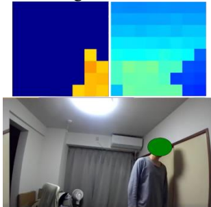
Fig. 9. Sensor output comparison: (A) AMG8833 (8×8 thermal) showing human signature, (B) VL53L5X (8×8 ToF) with distance data, (C) RGB reference (development only). Low-resolution sensors (A, B) enable reliable, privacy-preserving presence detection.
