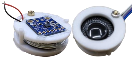
Fig. 4. Bottom layer of Garden Watch contains the audio subsystem (28mm speaker, MAX98357A amplifier) in a 3D-printed housing, supporting non-intrusive feedback for plant care and wellness checks.
