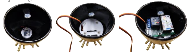
Fig. 7. Modular assembly of Garden Watch, stacking functional layers for easy installation and maintenance, ensuring serviceability and aesthetic, non-clinical design.
