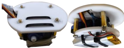
Fig. 5. Middle layer implementation showing the power and motion subsystems, including the LiPo battery (1000mAh), servo motor for nodding motion, and mini vibration motor for haptic feedback. This arrangement optimizes weight distribution while maintaining the garden ornament's aesthetic exterior.
