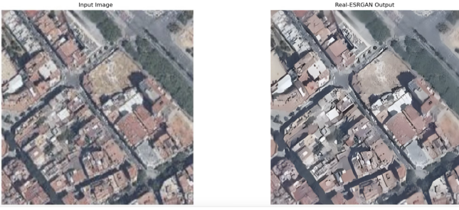
Fig. 3. Visual comparison of UAV image super-resolution. Left: Input LR image. Right: Output from Real-ESRGAN.
