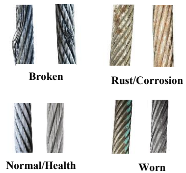
Fig. 2. Appearance of Elevator Steel Cable Condition
